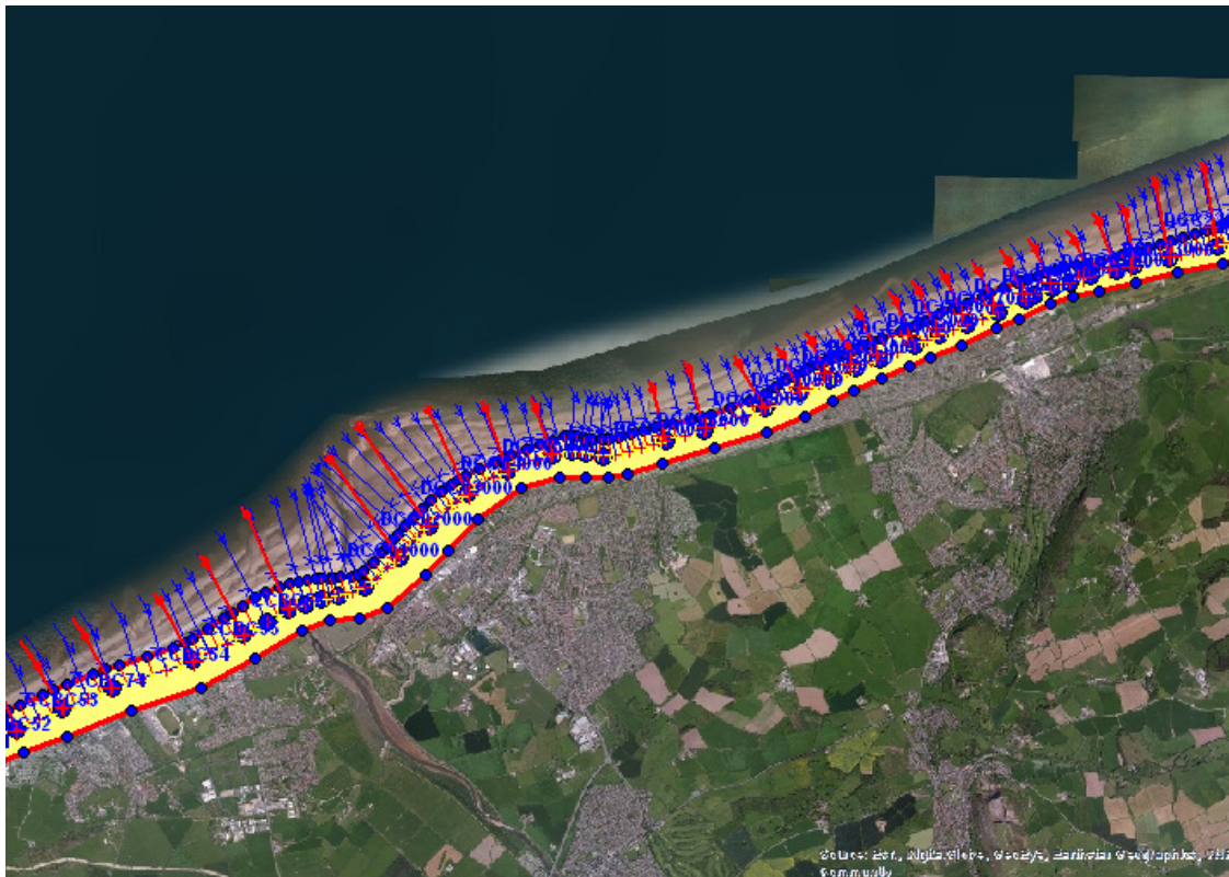
Figure 2-3: Illustration of Unibest profile density (blue lines), with comparison against measured profiles (red lines)
