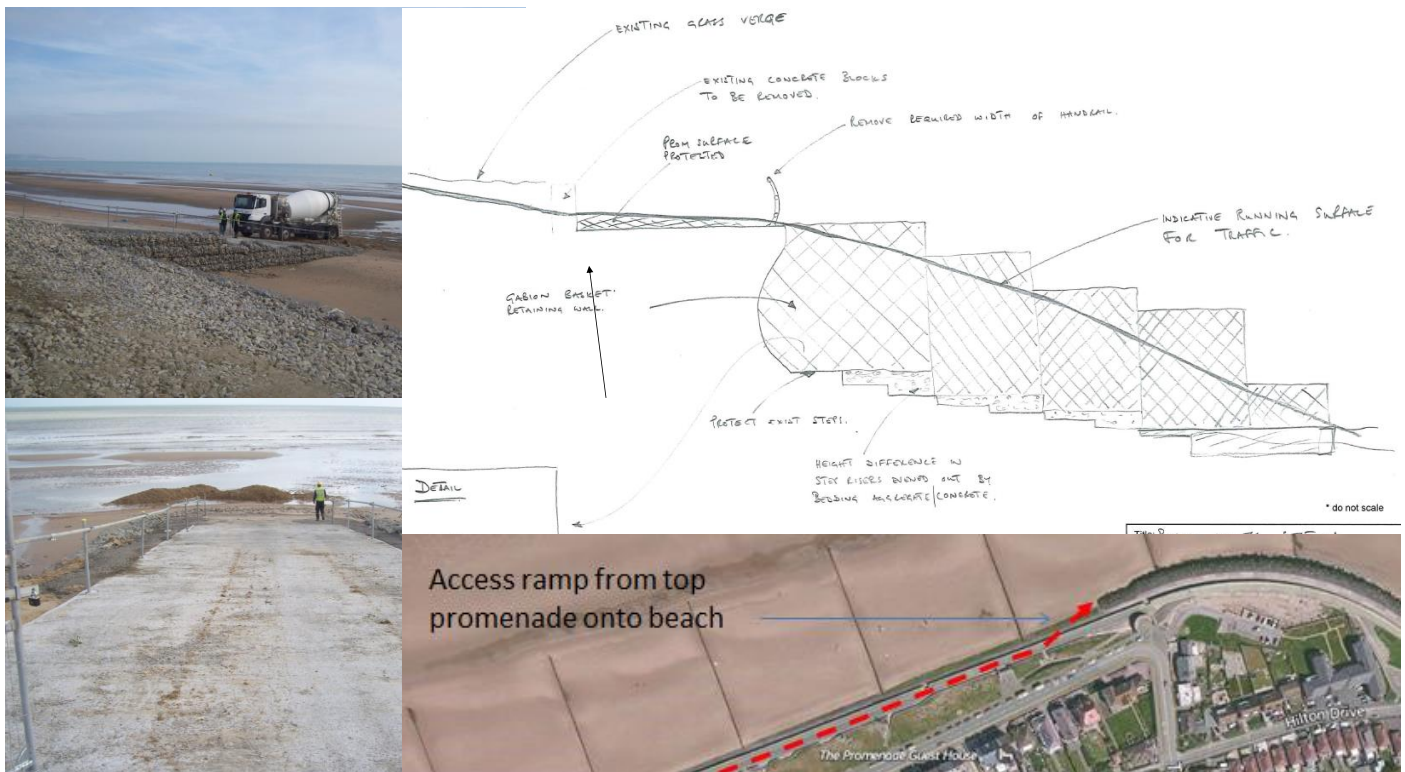
Figure 13- Temporary gabion retained slipway access near splashpoint
